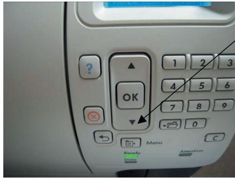
Once you have selected "Configure Device", press the down button on the display panel until it reads "Printing"
