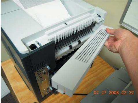
➤ The cover is not used while the PTM4515 is attached to the printer.
