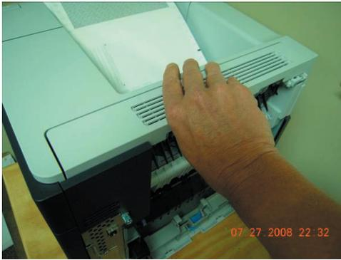
➤ Remove the cover from the top of the printer as shown. With the cover off, you will see a black connector on the top back left of the printer.
