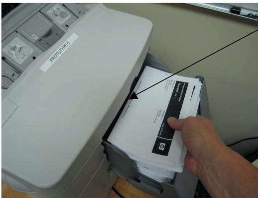
➤ It is also important to make sure that you do not interrupt the Exit Sensor located under the Hinged Top when emptying the Exit Tray
