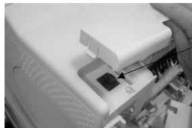
Remove the cover from the top of the printer as shown and store it for future use. With the cover off, you will see a black connector.
