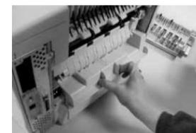
Next we will remove the paper feed tray dust cover. Simply grasp the cover in the center and pull out.
