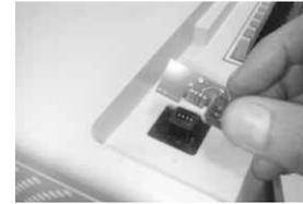
Leave the protective rubber band on the adapter board. This ensures that the adapter board is set correctly. Attach the Jetlink adapter board to the black connector on the top of the printer. Press gently to ensure a good connection, but not hard enough to cause damage to the connector or Jetlink connector board.
