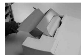
The hooks of the adapter should slip easily into the top chute opening of the PTM.
