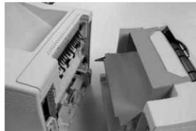
The adapter ramp has two spring tabs that engage the printer. Be careful not to damage or bend the spring tabs. They are critical for positioning the PTM with the printer. These spring tabs will be used to mate the PTM to the printer. Slide the PTM at an angle toward the printer with the right side going in first.
