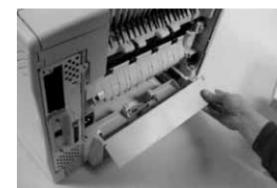
The pivoting feed tray cover is also easily removed. Lift the right side out of the snap. This allows the left side to slip out of the pivot hole in the paper tray. Store the pivoting tray cover with the rear door and dust cover in a safe place for future use.
