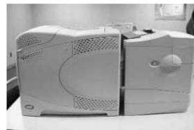
When finished, the printer and accessory should look like this. Notice the gap between the units to allow for paper movement and electrical connections.
