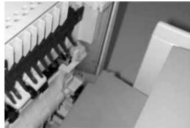
The right spring tab will slide inside the printer chassis into the opening in the printer where the rear door was removed. Be careful not to catch the spring tab on the printer side cover causing the spring tab to bend outward. Once the right spring tab is in place, continue sliding the PTM toward the printer.
