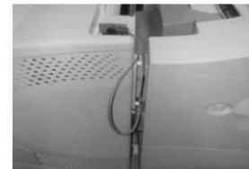
Once you have docked the PTM with the printer, the unit should be approximately  $\frac{3}{4}$ " away from the printer, with the adapter ramp firmly in place against the diffuser of the printer and the Jetlink cable plugged into the connector on the top of the printer.
