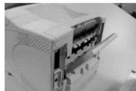
First, remove the rear door. The door drops down and is hinged.
